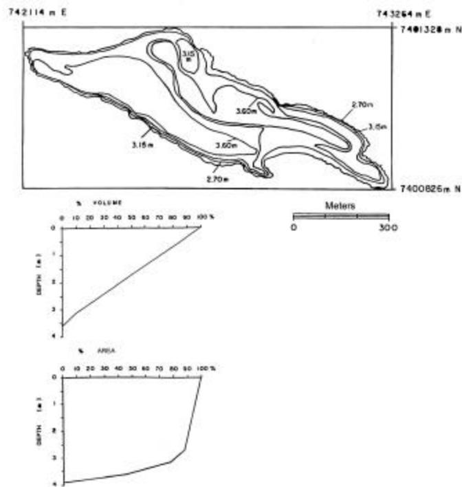
Figure 5: Batimetric map (above) and hypsographic curves (below) of volume and area of the Camargo Lake.
