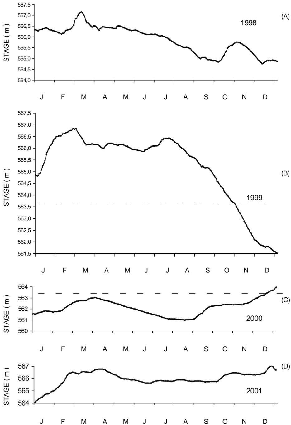
Figure 3: Daily water level variations (stage in m) at the dam of the Jurumirim Reservoir from January 01 to December 31 in 1998 (A), 1999 (B), 2000 (C) and 2001 (D). Dashed line represents the water overflow (when >563.60 m) between potamophase and limnophase.
