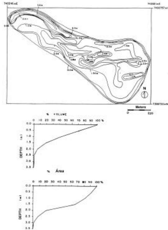
Figure 4: Batimetric map (above) and hypsographic curves (below) of volume and area of the Coqueiral Lake.
